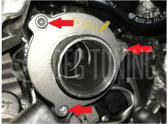
7. Carefully remove the stock O-ring from the turbo muffler.
