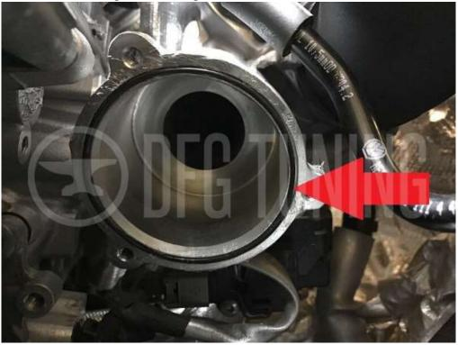
10. Install the DFG Turbo Muffler delete by holding it in place against the turbo housing while re-installing the (3) 5mm Allen bolts.
