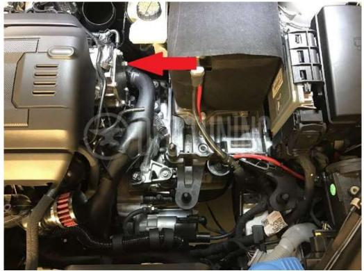
3. Loosen the two 7mm hose clamps that are attached to the Turbo Muffler
