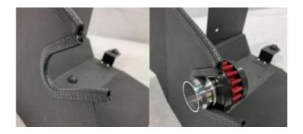
11. Assemble the intake tube using the rubber coupler and supplied clamps.
