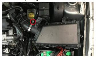
2. Now locate and remove the two 10mm bolts holding down the factory air box
