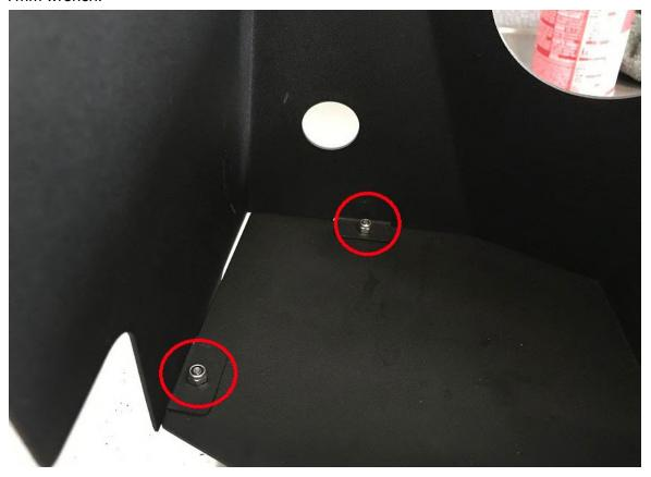
3. Locate the mounting tab and hardware (4mm allen wrench & 10mm locking nut) supplied with the intake system. Now install the mounting tab onto the intake as shown. Do not tighten down until after installation.
