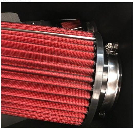
7. Now install the completed heat shield onto the vehicle by first pushing the intake tube onto the MAF sensor and tightening the clamp with a 7mm socket or flat head screwdriver.
