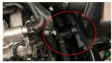
4. Locate the MAF (Mass Airflow Sensor) and unplug it by sliding the clip towards the hood and pulling up.
