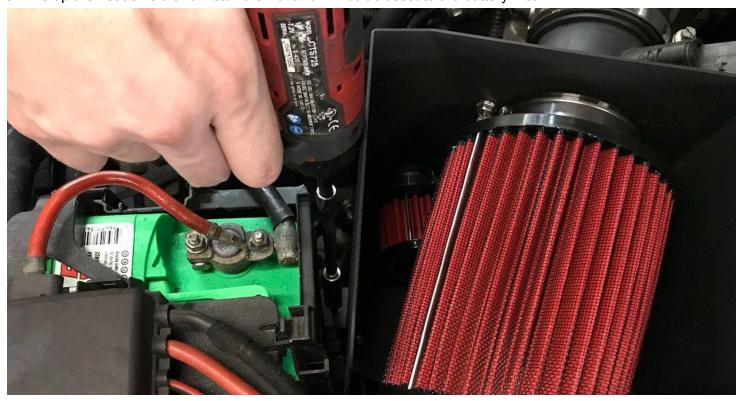
9. Now locate and install the 10mm bolt that connects the intake to the strut tower. Once installed you can tighten the 4mm Allen key bolt which connects the heat shield and mounting tab.
