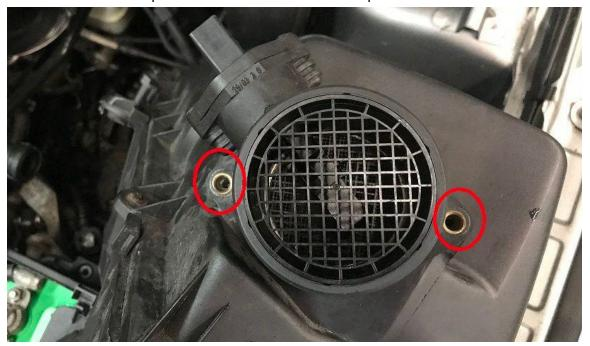
2. Now locate and assemble the DFG Tuning heat shield. To do this you will need the 2.5mm Allen key and 7mm wrench.
