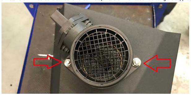
6. Now install the air-filter onto the MAF from inside the heat shield. Tighten down the clamp using a Phillips head screwdriver.
