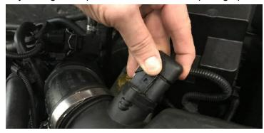
5. Lift the front of the intake box towards the engine to remove
