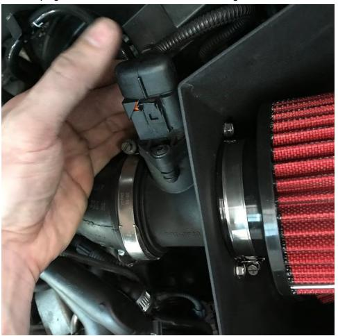
11. Re-install air pump tube onto the CNC adapter which is attached to the heat shield. You will hear it click into place.
