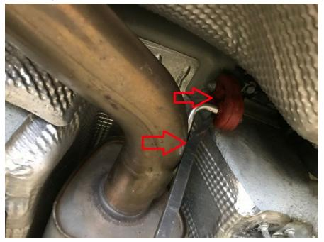
4. Have a friend hold the muffler or support the muffler using a jack
