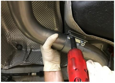
c. Once in the proper location tighten down the two clamps using a 15mm socket.
