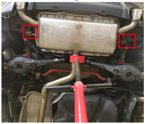
b. Remove the 13mm bolts on each side
