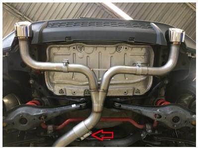
b. If you need more adjustment loosen the forward most compression clamp and move the pipe in or out to create the desired tip alignment.
