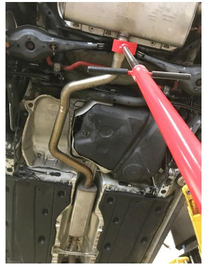
Once supported unbolt both rear exhaust hangers. Each hanger is held in place by a 13mm bolt
