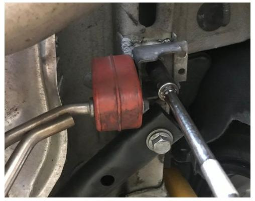
6. With the muffler now supported, loosen the center band clamp which is held on by two 13mm nuts and carefully remove the stock cat-back system
