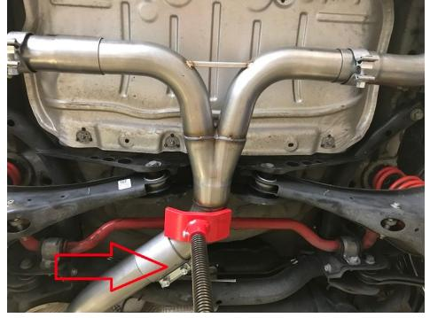
b. This will require two people as the system needs to be supported in the proper location as both sets of clamps are tightened down.
