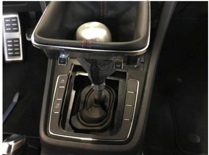
8. Slide assembled boot and shift knob on to shifter shaft and determine desired height.
