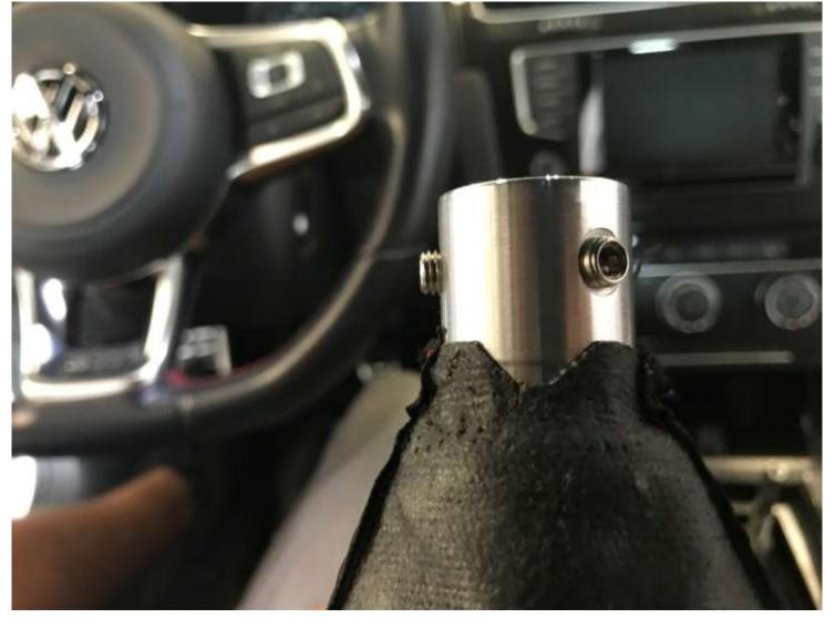
7. Line up the top of the boot with the bottom of knob that will be exposed, use the supplied zip tie to fasten the boot to the knob, be sure to smooth out any bunching of materials or undesired pinches, pull zip tie tight and snip off the excess zip tie/
