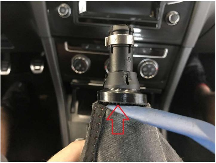
5. Once the collar is off, remove the shift knob from the shifter boot.
