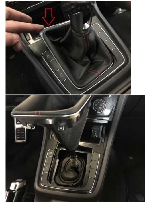
2. Locate and gently spread the locking collar with a pick tool or small flat head screwdriver
