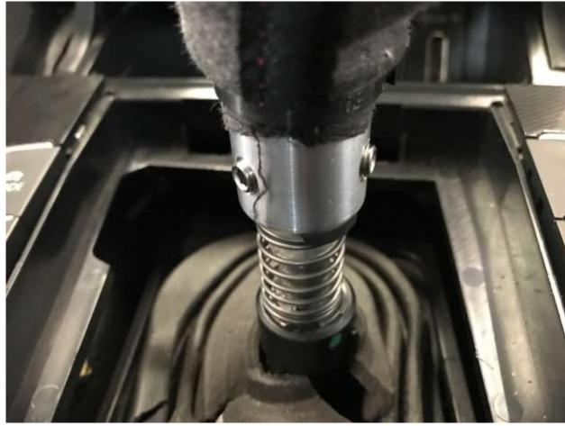
10. Push down the shift boot and reinstall the shifter trim.
