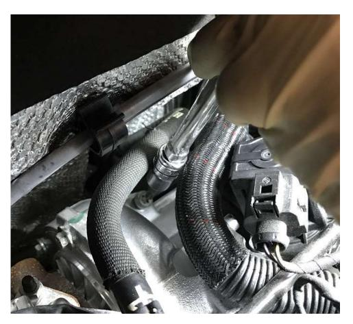
5. Now re install the PCV hose my pushing it back into place on the DFG Tuning inlet
