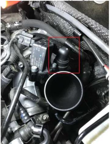
3. Now remove the stock turbo inlet by twisting the unit clockwise and pulling.
