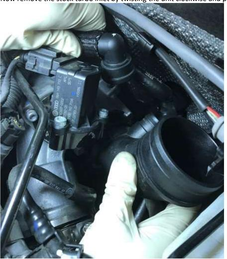
4. Once removed, transfer the O-ring from the stock turbo inlet to your new DFG Tuning turbo Inlet. Once installed on the DFG Tuning Turbo Inlet we recommend regreasing the o-ring before reinstalling it.
