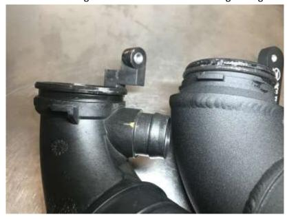
Now install your DFG Tuning Inlet by slowly placing the inlet in place and turning counter-clockwise to lock it in position. Once it is in the correct position, then you will be able to reinstall the T-30 screw.
