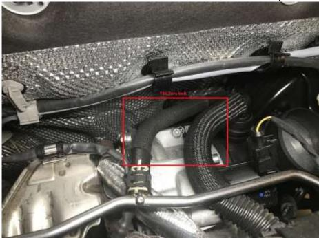
2. Now Remove the PCV vent hose by pulling up on the hose (This can require some force)
