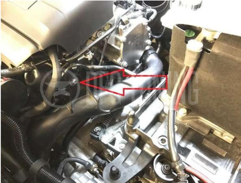
5. Remove the hose from the turbo muffler delete
